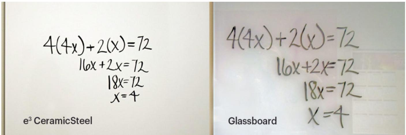
The text on the glass board is not as visible. The translucent nature of the surface is subject to reflection and glare causing distractions and potentially eyestrain to the user. Compare this to the image on the left. The CeramicSteel surface is clearly more visible and it is much easier for the observer to focus on the words rather than competing images caused by glare and reflections.
