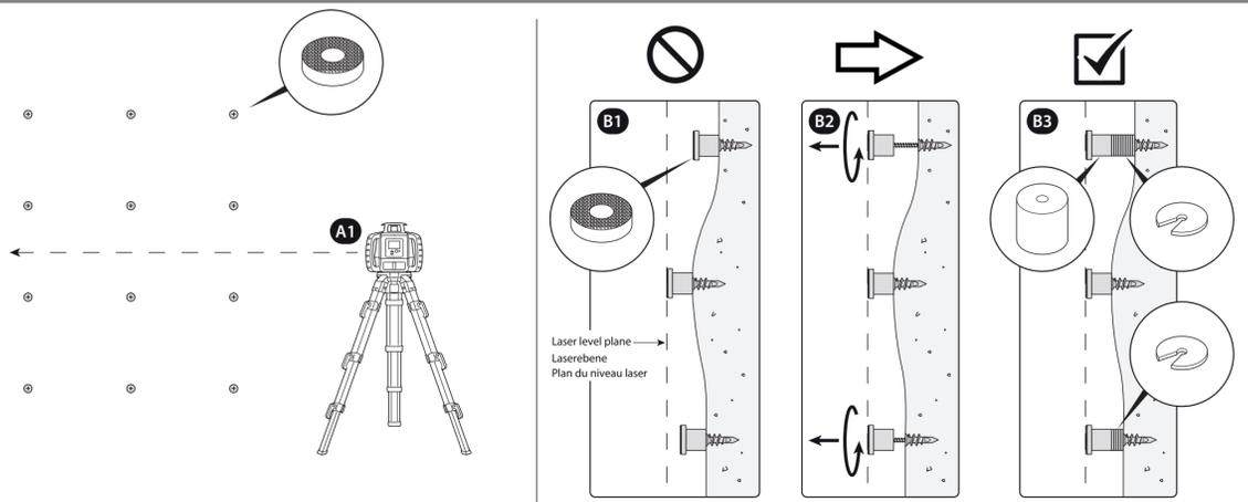
**A Set up laser level.** Project a laser plane parallel to the wall surface and as close to the wall as possible (A1). Using a tape measure or similar measuring tool, determine which dual lock hook location protrudes from the wall surface the most. Make a mark on the wall to indicate which location protrudes the most.
