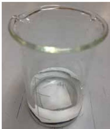
**17. Solvent test: toluene, methylethylketone, ethylalcohol, petroleum, grease, oil, ethylacetate or xylene (Dip 25 °C, 1.000 hours) | PVNV 41.822**
