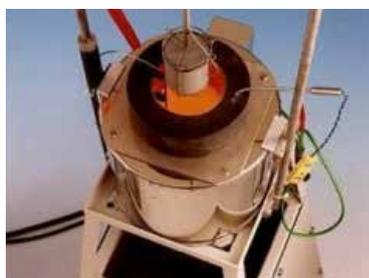
Reference norm/specification or document: EN 13501-1 +A1: references to (EN) ISO 1182 (Non-combustibility test) and (EN) ISO 1716 (Determination of the heat of combustion).
