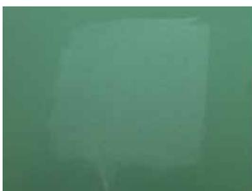
**Note:** Poor wet erased lab sample shown for illustration of ghosting
